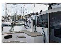
Out in the cockpit, the dual helm stations are positioned behind the saloon bulkhead, centralising weight and reducing motion, as well as giving you protection from the elements. You can sit on the coaming or stand at the wheel for excellent vision all-round, with the main and jib sheets positioned right in front of you and the traveller and spinnaker sheets close to hand.
